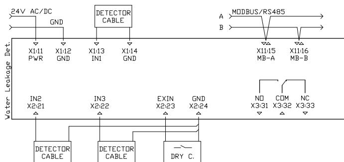
Relay contact rating is max. 1A at 230 VAC.
