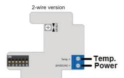
Important: connections in parallel with 24 VAC to consider the phase to prevent short circuits. The device is designed to operate in a low voltage condition.
